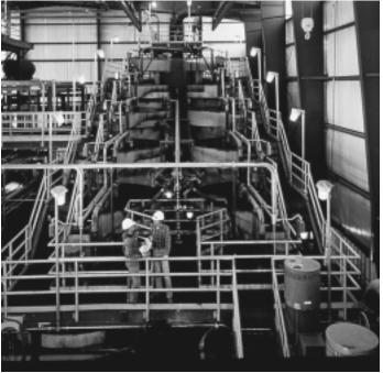
Gold recovery from cyanide solution using activated carbon (charcoal).
