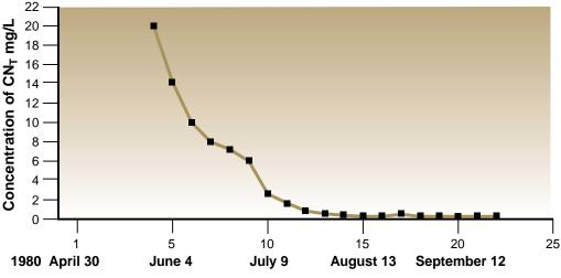
FIGURE 5. Example of Cyanide Degradation in a Shallow Pond
