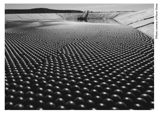
Floating "bird balls" cover the surface of a solution containment pond at the Cortez gold mine, a Placer Dome-Kennecott joint venture in Nevada, USA.
